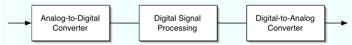
Figure 1: General Signal Processing Chain with a Digital Signal Processing Core
